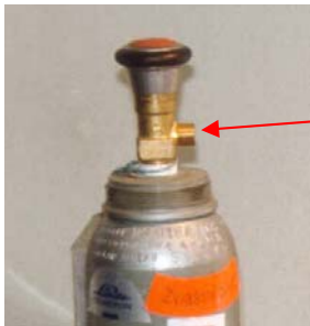
Fig.17.1- Calibration valve on gas cylinder
